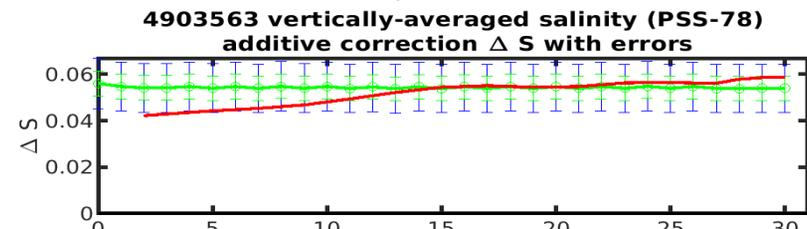
float profile number - blue: 2xcal error; green: 1xcal error; red: 1-1 profile f
