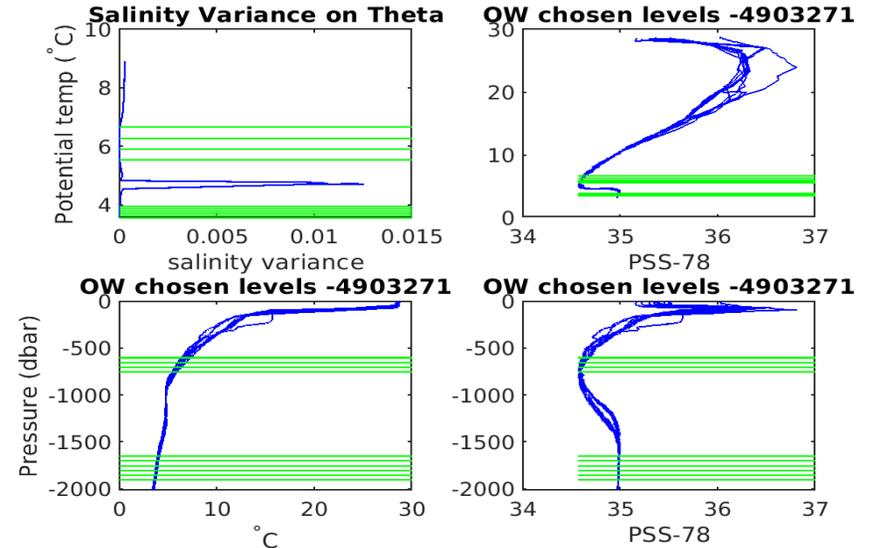
4903271 uncalibrated float data (-) and mapped salinity (o) with objective errors
