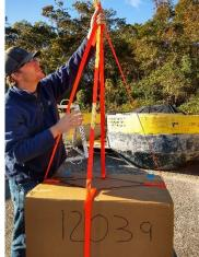
11. Attach a light line to the backup release, ensure that it doesn't get snagged.CAUTION: Pulling on or catching this line will pre-maturely release the float.
